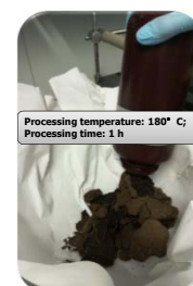
Fig. 2: Example of oven-dried hydrochar.
