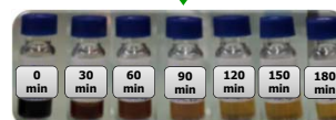
Fig. 1: Example of AHLs spilled in continuous at 220 °C and used for subsequent HPLC analysis.
